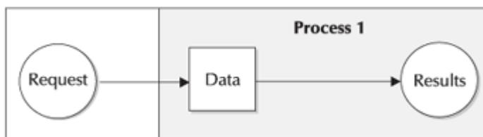
FIGURE 9-5. Serial processing
