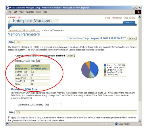
Fig 1: EM displays the current sizes of automatically tuned SGA components
